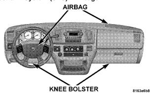
This vehicle has airbags for both the driver and right front passenger as a supplement to the seat belt restraint systems. The driver's front airbag is mounted in the steering wheel. The passenger front airbag is mounted in the instrument panel, above the glove compartment. The words SRS/AIRBAG are embossed on the airbag covers.
